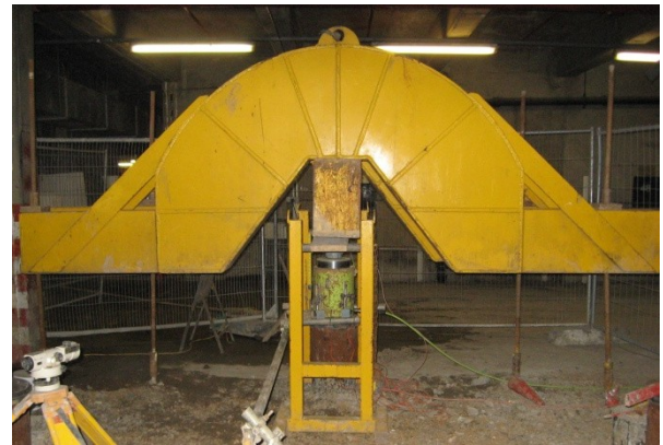
Figure 9 – Static Test Pile Reaction Framework
