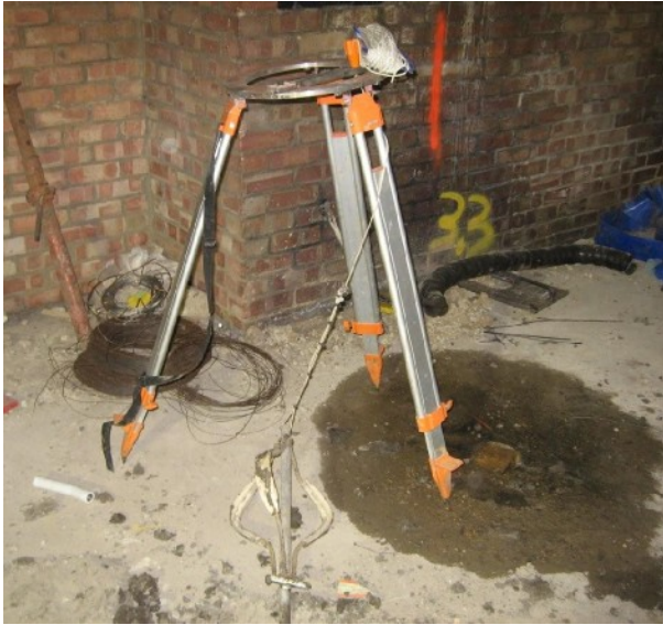
Figure 5 – Support Frame and Centralising Bracket
